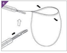
Place the desired specimen in the bag and pull out the handle placed on the outside while securing the bag with grasper to tie it.
